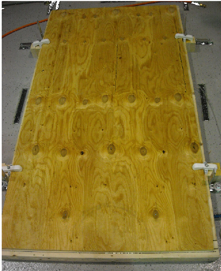
Figure 4: Frame with clamps fastened and plywood secured.
