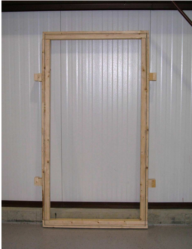
Figure 3: Window frame used for testing (Black lines indicate the area to be covered by plywood)
