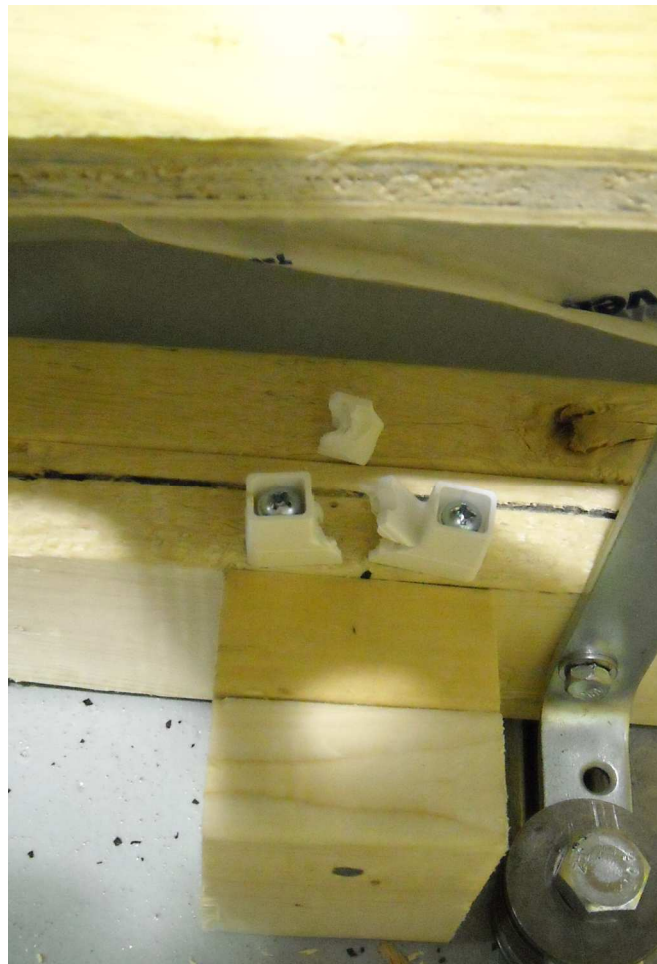
Figure 7: Failure of the clamp base during the uniform load.
