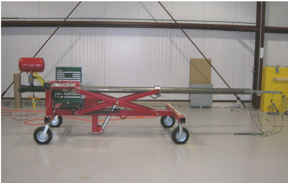
Figure 5: Air cannon apparatus used for launching large missile
